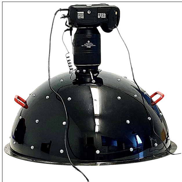
Figure 1: The CCeH RTI Dome with the Nikon D800 camera mounted on top.
